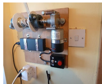
Hoisting a pulley full of clothes is impossible for clients with weak grips or arms. This modified windscreen wiper unit solves the problem.
