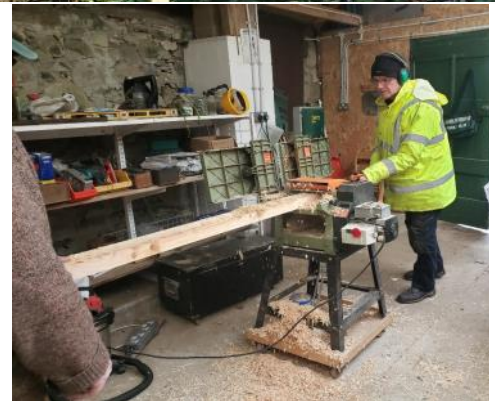
Pictured: Kirkdale Shedders Andy and Tony using a thicknesser to plane the wood for their bench into a uniform size.
